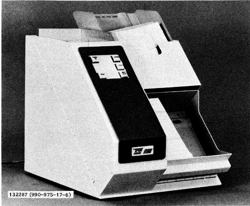
Figure 5-18. Model 804 Card Reader
